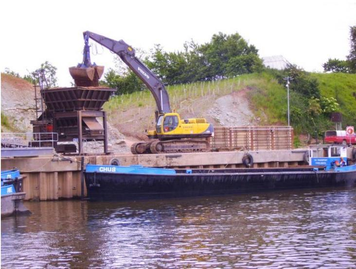
The aggregate is extracted from a quarry near Ripple and transported by barge two miles north to CEMEX's Ryall plant near Upton-upon-Severn, Worcestershire, with four to seven loads per day being moved. At Ryall the aggregates are washed and separated into various grades and delivered by road to CEMEX concrete making plants.
