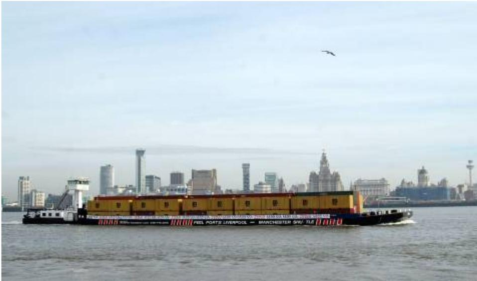
Peel Ports' Liverpool – Manchester Shuttle operated by a tug pushing a barge capable of carrying up to 160 20ft containers, runs weekly from the international container terminal at Liverpool to the Irlam Container Terminal 40 miles up the River Mersey and Ship Canal.
