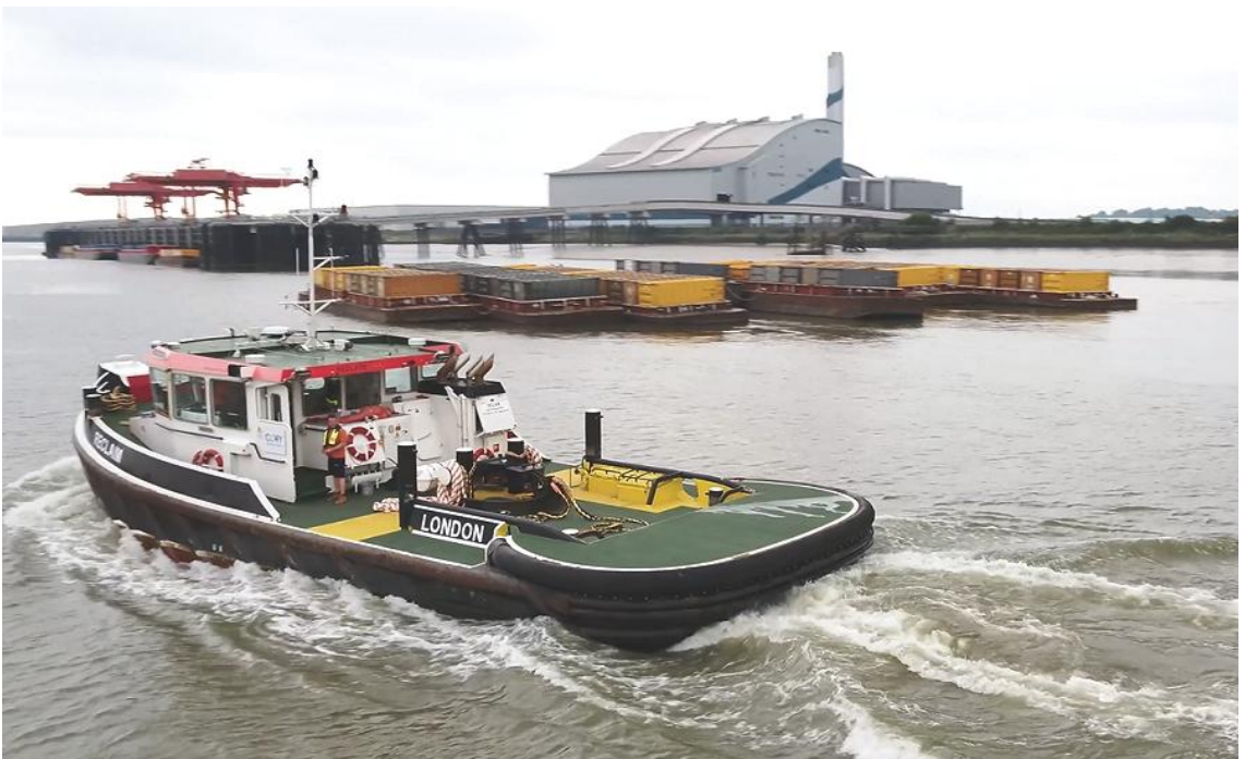
One of Cory's fleet of 5 tugs and 50 barges, carrying c.1 million tonnes of residual waste and aggregate per year to the Energy from Waste plant in the background (Cory Riverside Energy)
