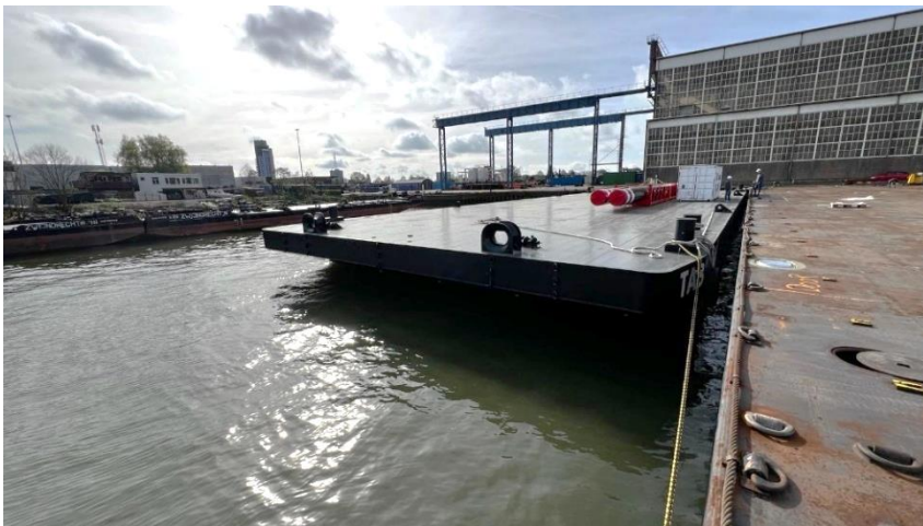
2024 built 50 x 18.8m barge – GPS 501 at delivery
