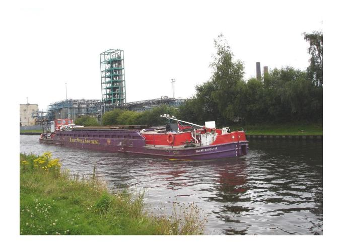
A current example is Exol Oils in Rotherham which brings imported oils by tanker barge from Hull – 460 tonnes a time; saving, as they say, not only 34 HGV lorry journeys a week but also vastly improving handling efficiency when deliveries arrive at their site. The barge – seen here in Rotherham - unloads in 6 hours; the equivalent number of lorries would take 17 hours
