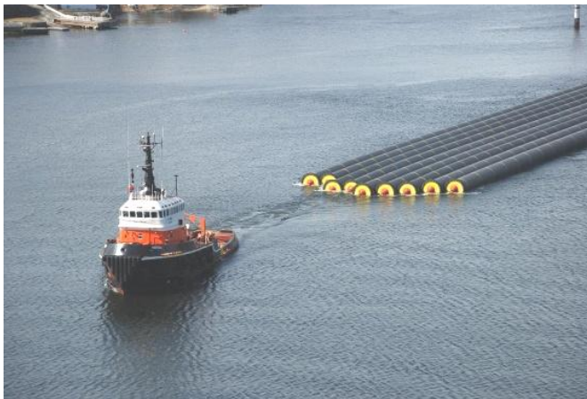
GPS Ocean going tug Hibernia towing pipes (GPS)
