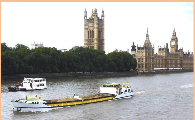
Barge carrying aggregate at Westminster, of the type envisaged for the Tunnel work (Thames Tideway Tunnel)
