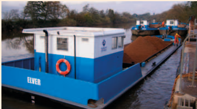
Converted at RWD Davies boatyard at Saul Junction the Elver went into service in 2008. With her squared off stern she can lift 15t more than her sister vessels.
