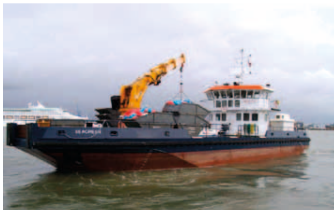
Veolia have taken delivery of a new barge to carry waste skips across Southampton Water to Marchwood. Nick MacWhirter’s innovative design for Seagreen provides the barge with self loading facilities. CBOA says the ability to load skips – a waste transfer unit in the waste management industry – is a welcome development.
