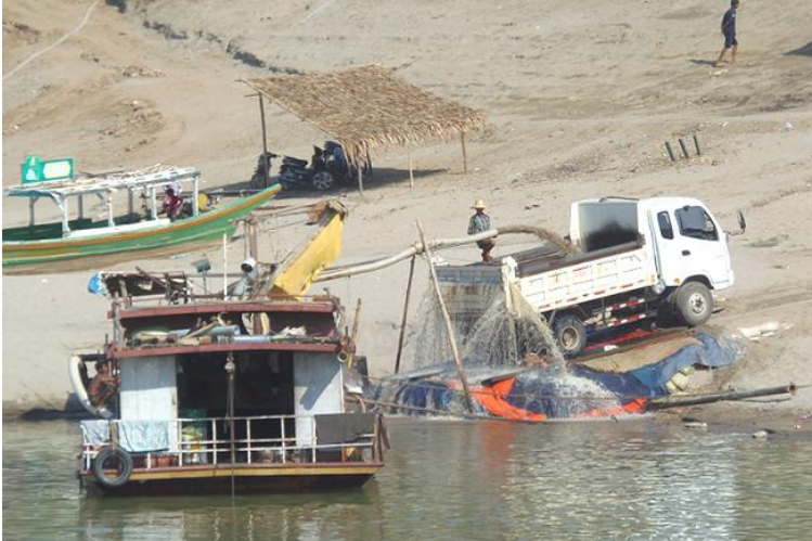
A suction dredger pumping out stone at Bagan – the lorry tailgate acting as a useful strainer (R Horne)
