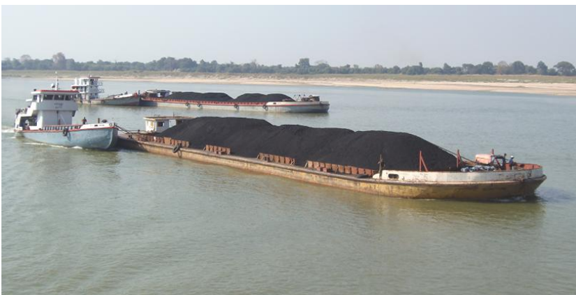
The coal pan in the foreground got free with the surge from being passed; the pan behind remained stuck (R Horne)
